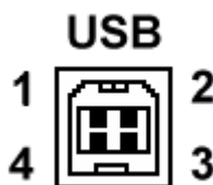
Figure 3-6: USB Connector pin orientation.
